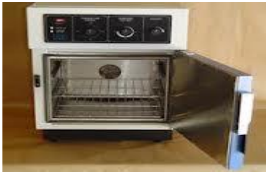
Gambar 16. Oven sterilisasi alat-alat gelas Sumber gbr, Organikganesha.com/bahan- alat.mini-lab
