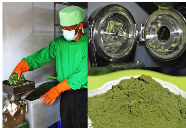
Flouring using stainless steel machine, and packaging with aluminum foil. Level of refinement reached to 200 mesh. Our packaging size of 250 g, 500 g, 1 kg, 5 kg, 10 kg, 20 kg.
