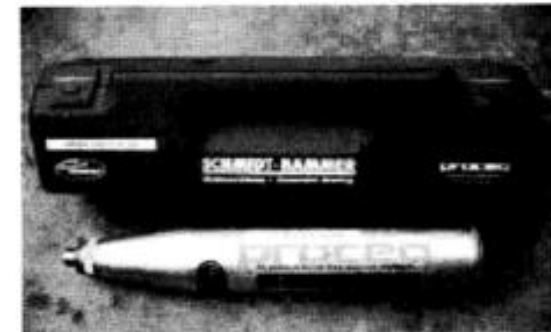
Gambar contoh alat Hammer Test
