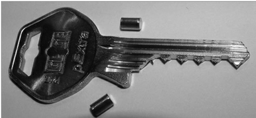
Figure 7-7: A typical bump key for a door.
