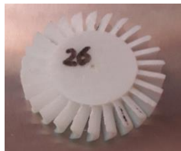
Gambar 2 Turbin impuls bidirectional
